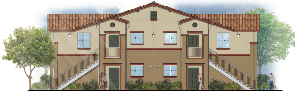
SIDE ELEVATION BUILDING 1 (opposite side similar) 3/16"=1'-0"
