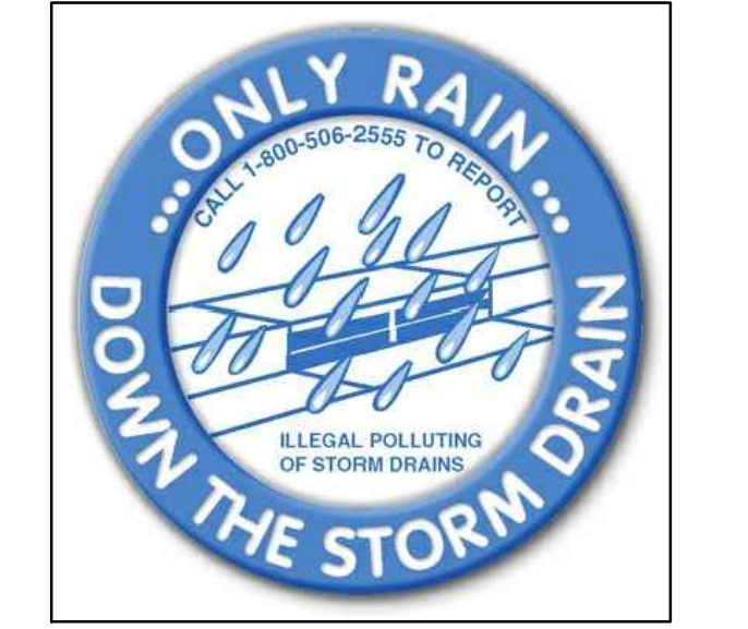
SAMPLE STENCIL TO BE USED NEAR GRATE AND CURB OPENING INLETS STORM DRAIN STENCILING N.T.S.
