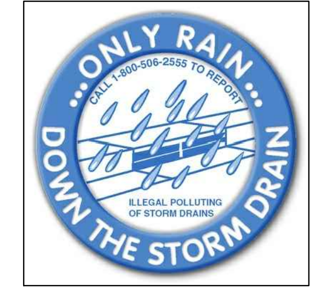
SAMPLE STENCIL TO BE USED NEAR GRATE AND CURB OPENING INLETS STORM DRAIN STENCILING N.T.S.
