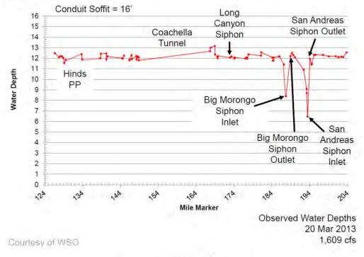
Figure 1 Observed Water Depths at Design Flow
