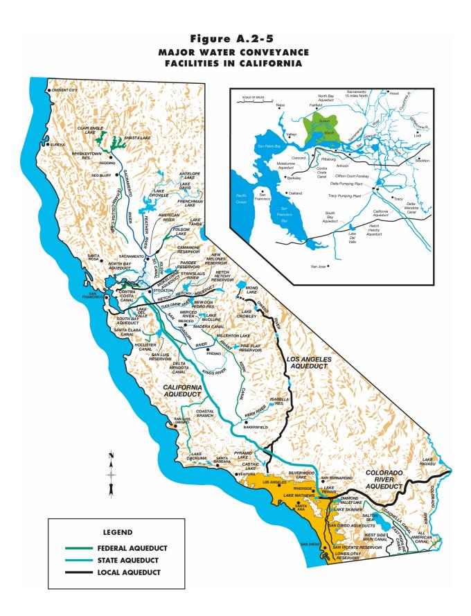
The water is delivered to Metropolitan's service area by way of the CRA, which has a rated capacity of approximately 1,700 cfs. The CRA conveys water 242 miles from its Lake Havasu intake to its terminal reservoir, Lake Mathews, near the City of Riverside. Conveyance losses along the CRA of 10 TAF per year reduce the amount of Colorado River water received in the coastal plain.
