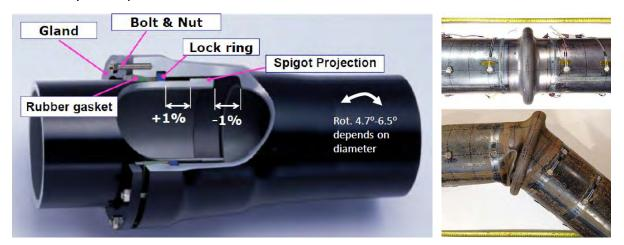
Figure 4-2: Example of Seismic Resistant Pipe (courtesy of Kubota Corp. and JFE)
